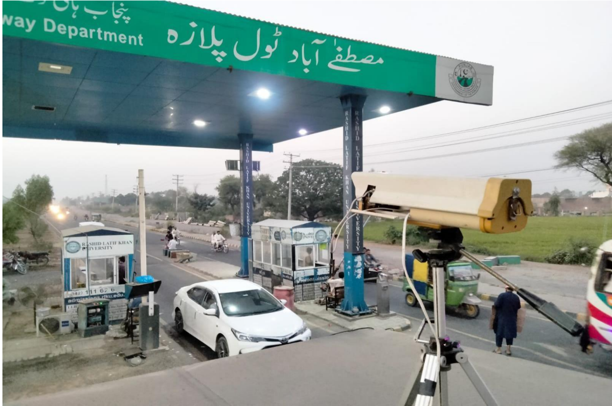
Figure 2 - Vehicle Counting Device Mounted at Traffic Survey Site
